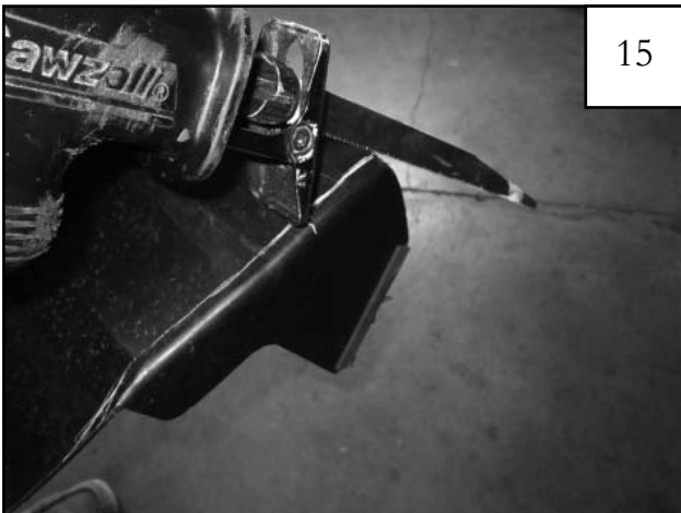
On front end of splash shield using a grease pencil and mark in 1/2" from the radius of splash shield and drawn a line till flush with outside edge of shield. Using a sawsall cut off section of splash shield where indicated.
