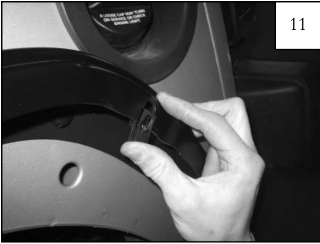
Install supplied "U" Nut, with the thread side in, over holes in Inner Flare Piece (8 places).
