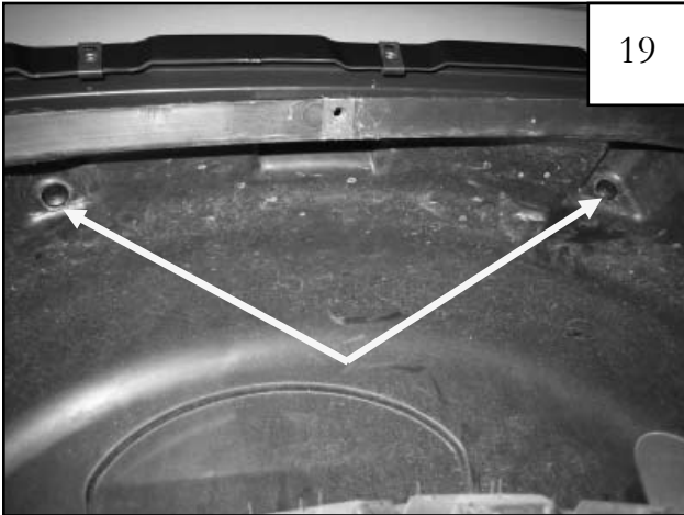
Position splash shield in wheel well, and install two supplied Plastic Phillips Head Tuflocs in upper pockets using a pushing-twisting motion.
