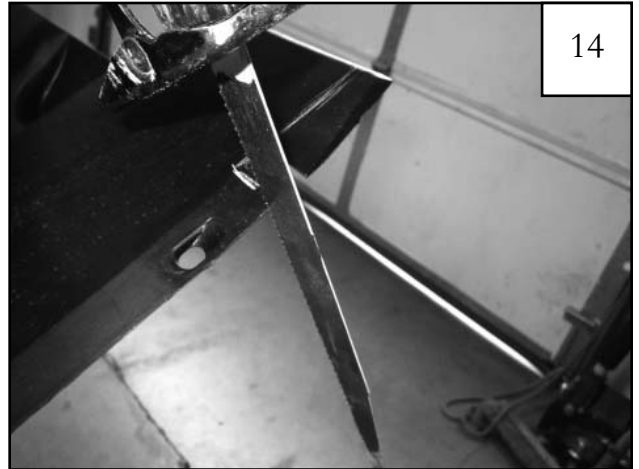
On rear end of splash shield using a grease pencil, measure in from last hole 1-1/4" and make a line from the edge of shield to style line. Then create a line from the style line out to the end of the splash shield as shown. Using sawsall to cut off section marked.
